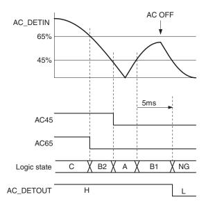
When the AC\_DETIN pin voltage does not rise to 65% or more of the AC\_VRMS pin voltage within 5ms after the state transitions to "B1", AC OFF is judged, the state transitions to "NG", and AC\_DETOUT outputs Low.
