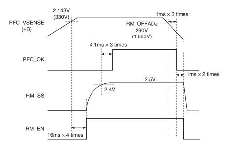
Fig. 4. PFC\_OK Signal Output Sequence
