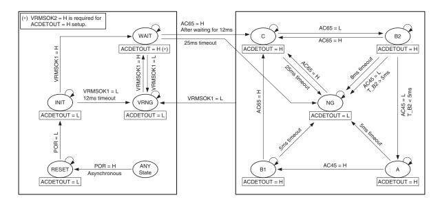
Fig. 2-2. AC Detection State Transition Diagram
