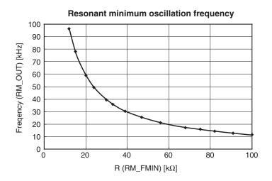
Fig. 14. Minimum Oscillation Frequency Setting
