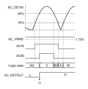
When the AC\_DETIN pin voltage rises to 65% or more of the AC\_VRMS pin voltage while the AC\_VRMS pin voltage is 1.75V or more in the "NG" state, the state transitions to "C", AC\_DETOUT outputs High, and the normal state judgment cycle starts. (t1)
