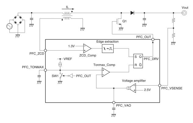
Fig. 5. Operation Circuit Block Diagram
