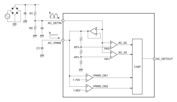
Fig. 2-1. AC Detection Block Equivalent Circuit
