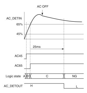
When the AC\_DETIN pin voltage does not fall to 65% or less of the AC\_VRMS pin voltage within 25ms
