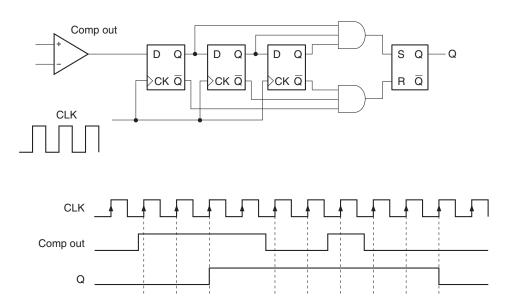
Fig. 1. Equivalent Circuit Corresponded to 1ms  $\times$  3 Times
