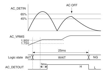
When the AC\_VRMS pin voltage is 1.95V or more but the AC\_DETIN pin voltage has not reached 65% of the AC\_VRMS pin voltage (the state has not transitioned to "C") within 25ms after the state transitions to "WAIT", AC OFF is judged, the state transitions to "NG", and AC\_DETOUT outputs Low.
