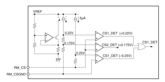
Fig. 17. Overcurrent Detection Block Equivalent Circuit
