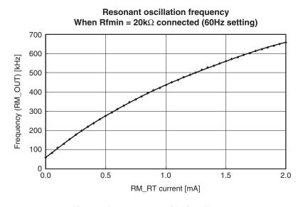
Fig. 12. Resonant Oscillation Frequency
