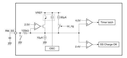
Fig. 15. Resonant Soft Start Circuit Block Equivalent Circuit
