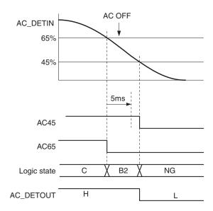
• When 5ms or more have elapsed by the time the AC\_DETIN pin voltage falls to 45% or less of the AC\_VRMS pin voltage after the state transitions to "B2", AC OFF is judged, the state transitions to "NG", and AC\_DETOUT outputs Low.
