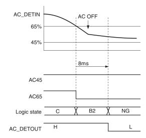
When the AC\_DETIN pin voltage does not rise to 65% or more or fall to 45% or less of the AC\_VRMS pin voltage within 8ms after the state transitions to "B2", AC OFF is judged, the state transitions to "NG", and AC\_DETOUT outputs Low.
