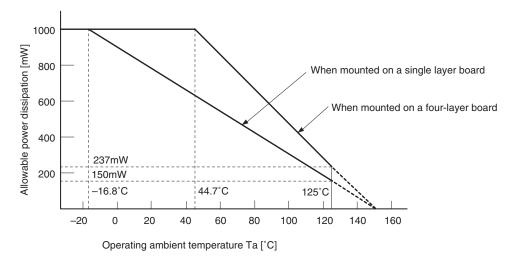
Glass fabric base epoxy board,  $76\text{mm} \times 114\text{mm}$ , t = 1.6mm
