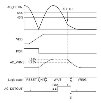
• When the AC\_VRMS pin voltage falls to 1.75V or less in the "WAIT" state, AC OFF is judged, the state transitions to "VRNG", and AC\_DETOUT outputs Low (t1).
