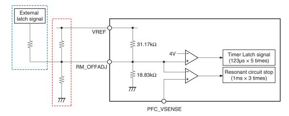
Fig. 20. RM\_OFFADJ Pin Internal Equivalent Circuit
