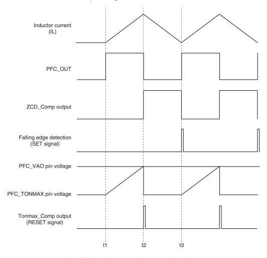
Fig. 6. Switching Operation Block Waveforms
