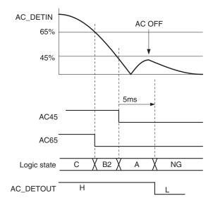
When the AC\_DETIN pin voltage does not rise to 45% or more of the AC\_VRMS pin voltage within 5ms after the state transitions to "A", AC OFF is judged, the state transitions to "NG", and AC\_DETOUT outputs Low.
