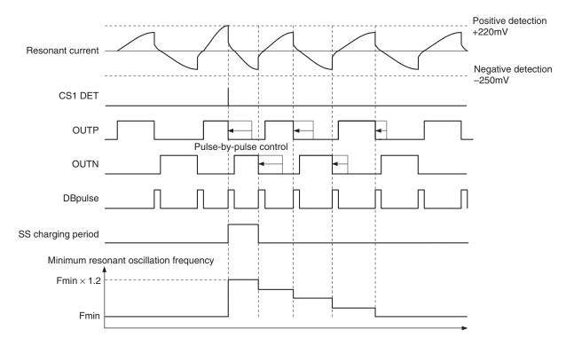
Fig. 18. Operating Waveform in Overcurrent Detection Mode
