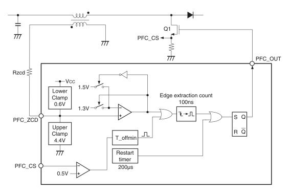
Fig. 7. ZCD Control Block Equivalent Circuit
