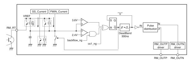
Fig. 11. Resonant Oscillator Equivalent Circuit
