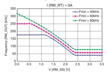
Fig. 16. Resonant Oscillation Frequency during Soft Start
