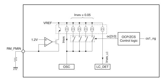
Fig. 13. Minimum Resonant Frequency Control Block Equivalent Circuit
